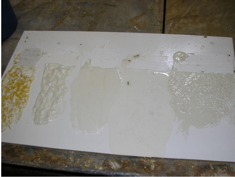
Figure 3-12. Panel After Three Hours of Stripping at Strip Joint
