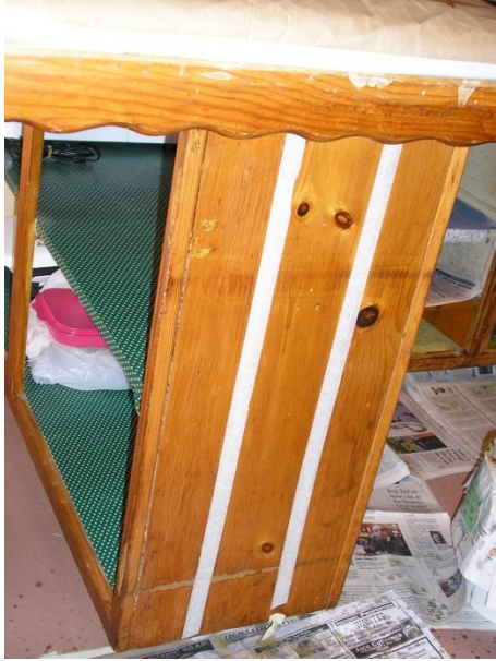
Figure 3-19. Panel #1 After Stripping
