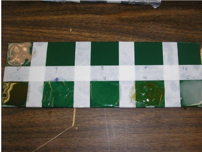
Figure 3-24. Green Metal Panel After Strippers Applied
