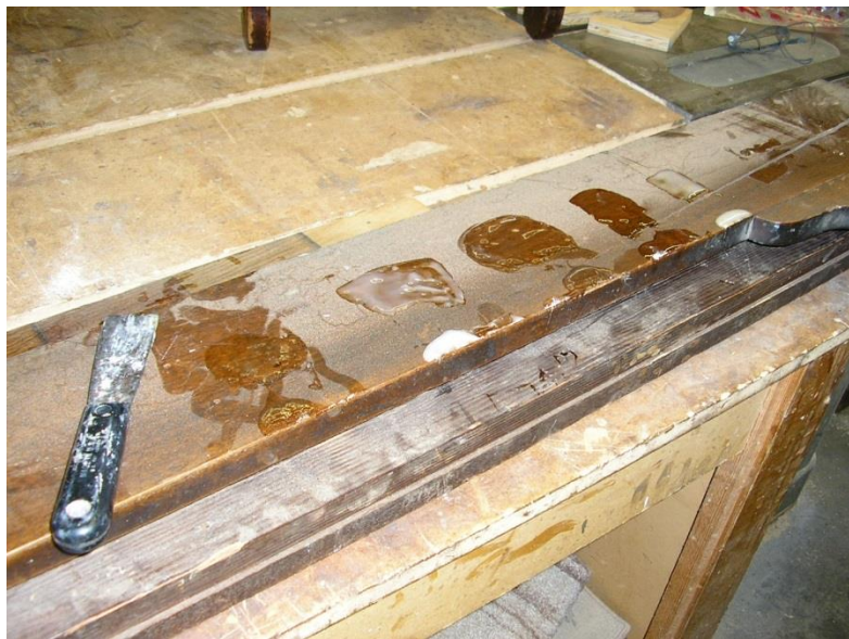
Figure 3-8. Bed Rail After Applying Five Strippers at Sunset Strip
